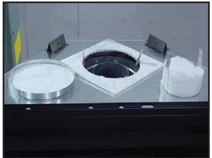
Figure 7.5 Discard the vent cap, remove and discard the insulation basket. Note: Once the vent cap has been removed it cannot be reattached.
